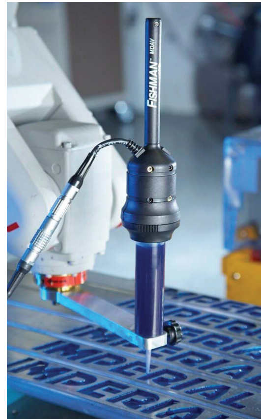
Figure 3. Fishman LDS9000 Dispense Gun Mounted in Robotic Arm
