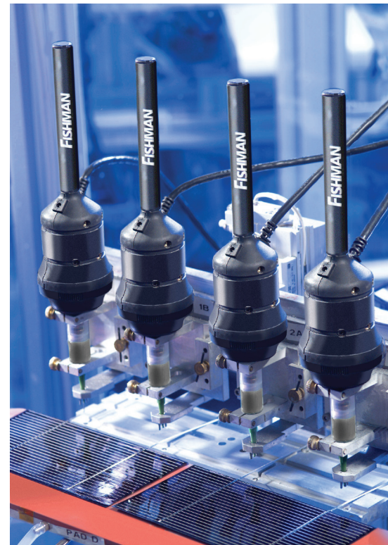
Figure 1. Evergreen selected four AirFree™ LDS9000 dispensing guns from Fishman Corporation. They are mounted side by side in a housing to optimize assembly line throughput.
