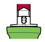
7.4 Holding both barrel reservoir and dispense gun loosely, step on the foot pedal until the barrel reservoir ears are raised at least 1/4" (6.35 mm) above the plate.
