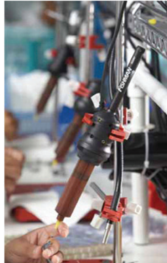
Production Line with Fishman LDS9000 Dispensing Systems Assembling Medical Devices
