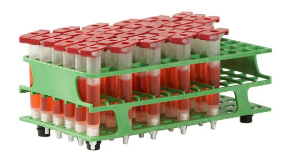
The SmartDispenser® syringe holding rack allows an operator to pre-fill dozens of syringes in one sitting and store them for future use. This accessory helps provide a clean, efficient and organized work station.
