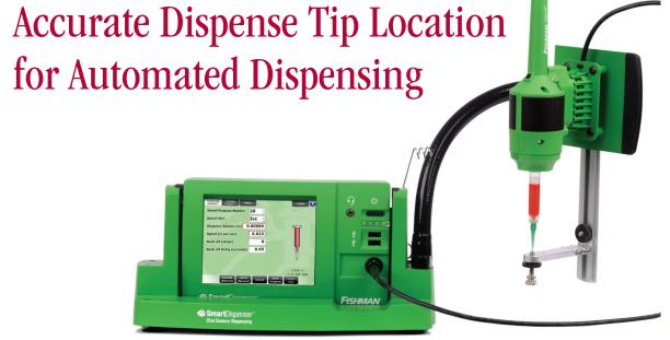
The dispense tip locator is part of the SmartDispenser® Priming Station. The dispense tip locator is attached to the back of the priming station gun stand. The locator provides a positive stop to assure the dispense tip is set at the proper height for fully automated assembly systems.
